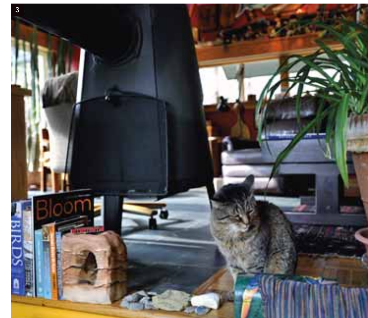
3. The living room's slate floor is made from salvaged high-school blackboards. Its dark gray color absorbs the solar energy that streams through south-facing windows, and the warmth is stored by the home's foundation—a system that's clearly cat-approved.
